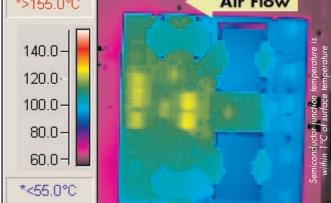
*Figure 8:* Thermal plot of converter at 12 amp load current with 55°C air flowing at the rate of 200 LFM. Air is flowing across the converter from output to input (nominal input voltage).
