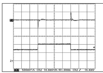
**Figure 12:** Output voltage response to step-change in load current (50%-75%-50% of Iout(max):  $dI/dt = 5A/\mu s$ ). Load cap:  $480\mu F$ , 15 m $\Omega$  ESR tantalum capacitor and  $1\mu F$  ceramic capacitor. Top trace: Vout (500mV/div), Bottom trace: Iout (5A/div).
