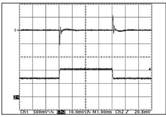
**Figure 11:** Output voltage response to step-change in load current (50%-75%-50% of lout(max);  $dI/dt = 0.1A/\mu$ s). Load cap:  $15\mu$ F, 450 m $\Omega$  ESR tantalum capacitor and  $1\mu$ F ceramic capacitor. Top trace: Vout (500mV/div), Bottom trace: lout (5A/div).
