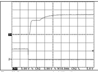
Figure 10: Turn-on transient at zero load (10 ms/div). Top Trace: Vout (5V/div) Bottom Trace: ON/OFF input (5V/div)
