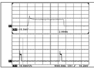
**Figure 18:** Load current (10A/div) as a function of time when the converter attempts to turn on into a 1 m $\Omega$  short circuit. Top trace (2ms/div) is an expansion of the on-time portion of the bottom trace.
