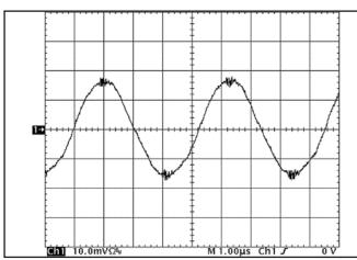
**Figure 14:** Input Terminal Ripple Current,  $i_c$ , at full rated output current and nominal input voltage with  $10\mu$ H source impedance and  $47\mu$ F electrolytic capacitor (100 mA/div). (See Figure 13)
